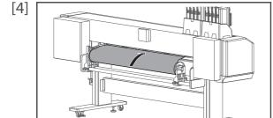
From the rear side of the printer, insert the front edge of the media into the media slot.
